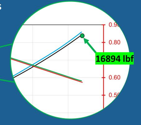
Thrust required is **lower** throughout powerband with lighter hardtop i.e. <u>Fuel is saved</u>
